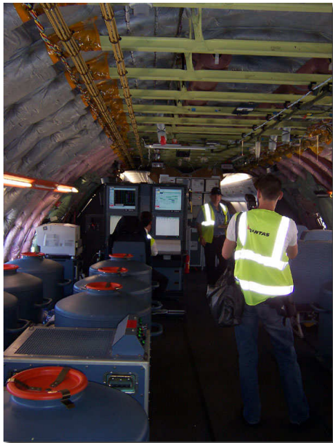
The upper deck of the A380, showing the ballast tanks and engineers station
