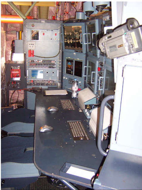
The engineer's station where all of the systems are monitored during testing
